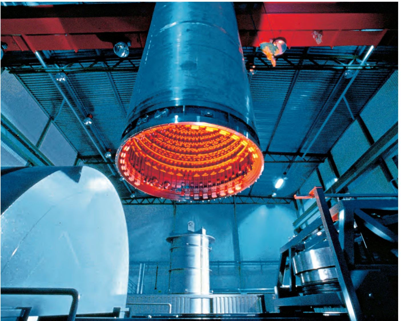
Figure 44. HIP mantle being lowered into place. © Bodycote
