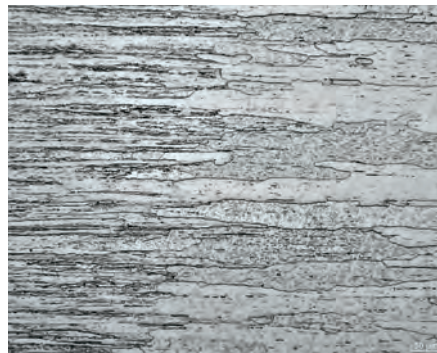
Figure 57. Transition between HAZ (right) and base metal (left) in TIG-welded ODS Mo-La alloy. © Rhenium Alloys
