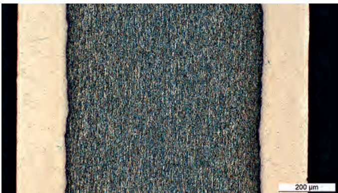
Figure 22. A “composite-composite” structure showing a MoCu core and a copper surface layer. © Plansee SE
