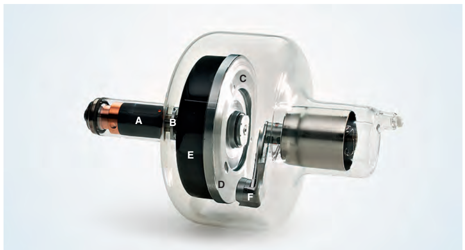
Figure 30. X-ray target showing rotor (A), stem (B), and molybdenum-alloy target (C) with tungsten-rhenium alloy track (D) for X-ray generation. Also shown are the graphite heat sink (E) and cathode cup (F) that contains the tungsten filament. © Plansee SE (X-ray tube produced by Dunlee)
